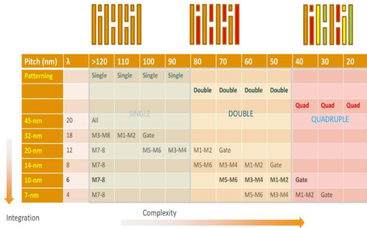
Figure 3.8: Single, double and quadruple patterning applied in the layers of advanced technology nodes
