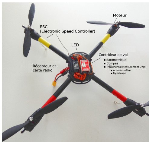
FIGURE 2.2 – Composants d'un drone.
