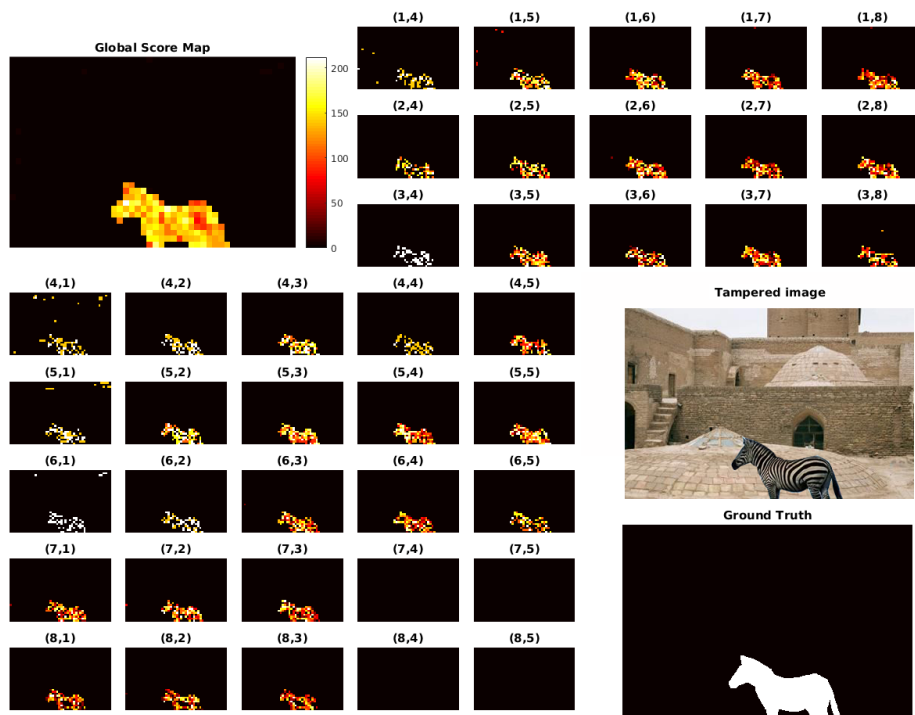
Figure 5.11: Individual score maps (small), the global score map (big, top-left corner), and forged image and its ground truth (big, bottom-right corner).
