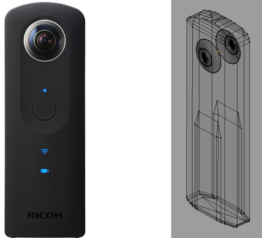
Figure 3.6 – Picture of the 360° camera. A simple 3D model of the reference object we use (created with blender): 303 vertices, 605 edges, 306 faces).
