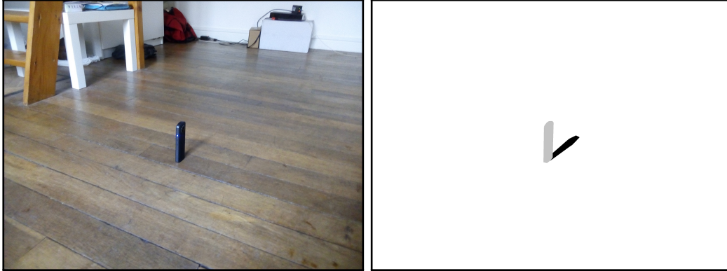
Figure 3.3 – Local scene containing the reference object and the shadow corresponding to the light source of the environment map (left). Mask of the shadow and of the reference object (right).
