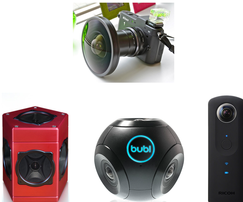
Figure 2.4 – Top: a fish-eye lens mounted on a camera. Bottom: Different 360° cameras (from left to right): Ladybug, Bublcam and Ricoh Theta.
