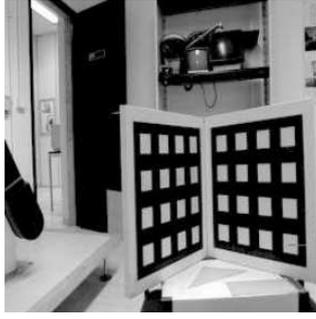
Fig. 2.2 Multi-planar chessboard 3D reference object-based calibration, source: [85].
