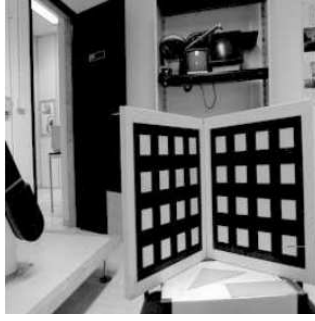
Fig. 2.2 Multi-planar chessboard 3D reference object-based calibration, source: [85].
