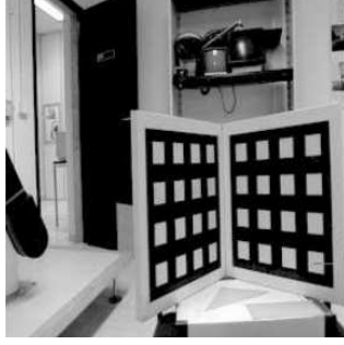
Fig. 2.2 Multi-planar chessboard 3D reference object-based calibration, source: [85].
