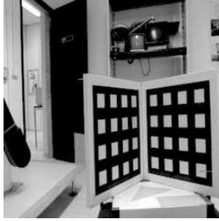
Fig. 2.2 Multi-planar chessboard 3D reference object-based calibration, source: [85].
