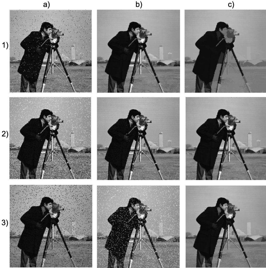
Figure 2.5: Filtering experimentation by a tree of shapes \phi and a component-trees (max-tree \tau^{max} and min-tree \tau^{min} ). 1.a) 2D image I with a 257 \times 258 pixels spatial resolution, [0, 255] gray levels and “salt and pepper” noise of 0.02 density. 1.b) and 1.c) filtered images reconstructed from \phi(\Theta(\text{area})) > \varepsilon_{\text{area}}\{20, 600\} . 2.a) and 2.b) filtered images from \phi(\Theta(\text{cont}_{\text{ext}})) < \varepsilon_{\text{contrast}}\{100, 140\} . 2.c) Fused area & contrast bi-conditioned filtered image from \phi(\Theta(\text{area})) > \varepsilon_{\text{area}}\{10\} & \phi(\Theta(\text{cont}_{\text{ext}})) < \varepsilon_{\text{contrast}}\{140\} . 3.a) and 3.b) filtered images from \tau^{max}(\Theta(\text{area})) > \varepsilon_{\text{area}}\{20\} and \tau^{min}(\Theta(\text{area})) > \varepsilon_{\text{area}}\{20\} , respectively, and 3.c) image result of these last two filtering processes sequentially applied in their appeal order.
