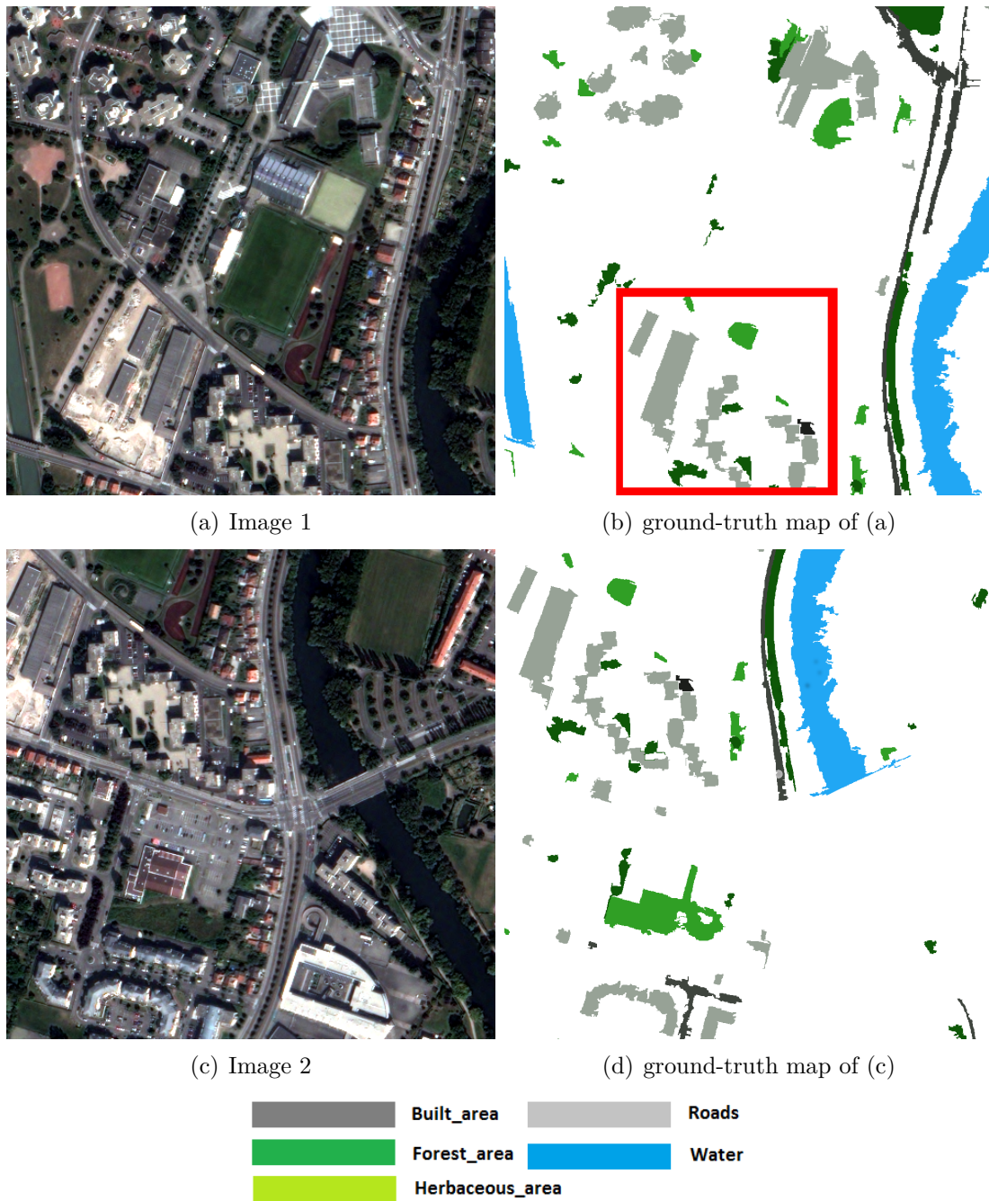
Figure 8.1: (a, c) VHSR images of 1000 \times 1000 pixels at a spatial resolution of 60 cm. (b, d) Ground-truth maps with reference segments belonging to 5 (coloured) semantic classes.
