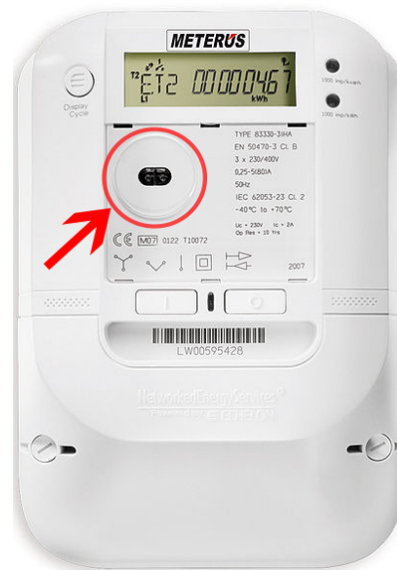
Figure 25: A power meter with an optical port (source: https://nl.wikipedia.org/wiki/IEC_62056 )
