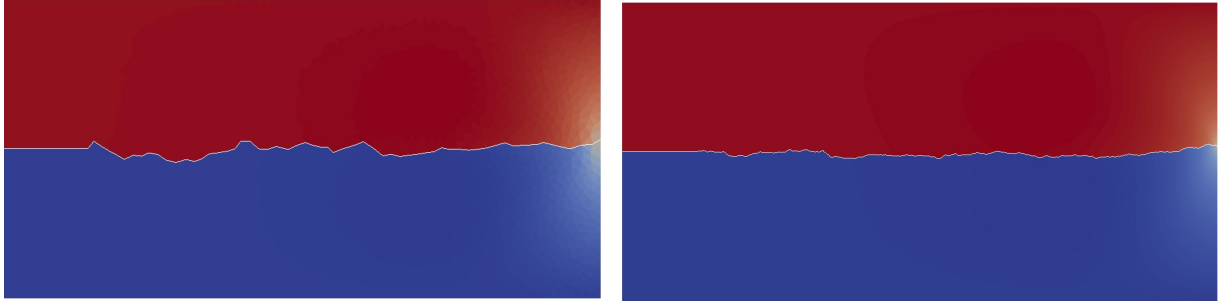
Figure 4.22 – Mode 1 (quasi-static): crack path on unstructured meshes.
