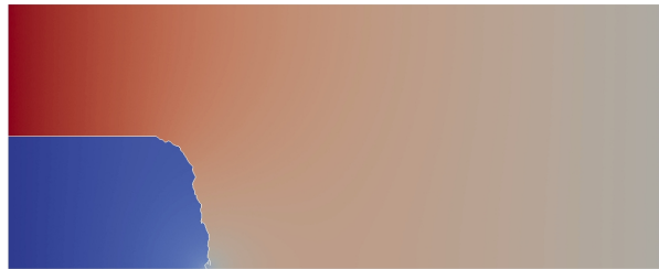
Figure 4.15 – Crack path computed with the kinking criterion (4.38) with an unstructured mesh containing a straight line.
