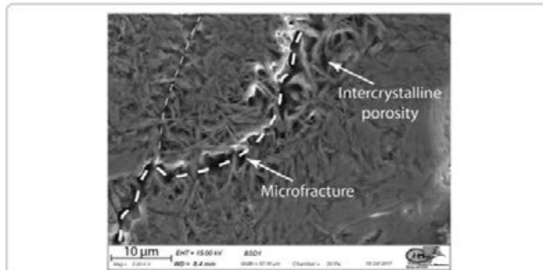
Fig. 5 Scanning Electron Microscopy (SEM) image of a small zone of altered sample 15.142 showing a total replacement of primary volcanic minerals and groundmass by K-phyllosilicates. Crystallization of K-phyllosilicates is posterior to the development of microfractures as they partially bond them. Intercrystalline porosity is also encountered between K-phyllosilicate crystallites
