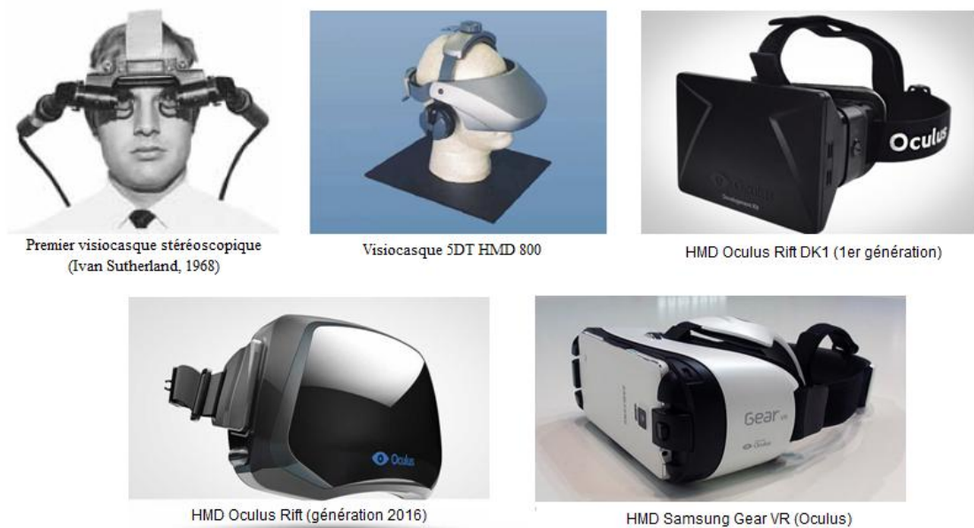
Figure 2-2. Evolution des Visiocasques ou HMD (Head Mounted Display).
