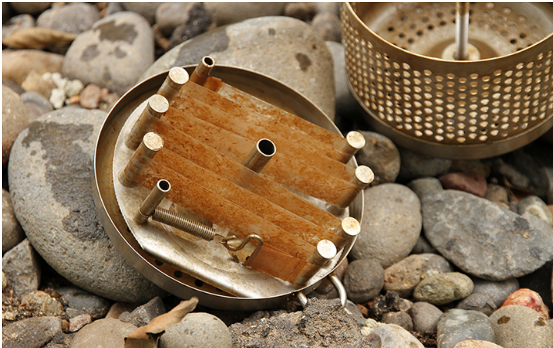
Image 7: SPMD (Semi permeable membrane device). (crédit photo. S. Becerra, 2013)
