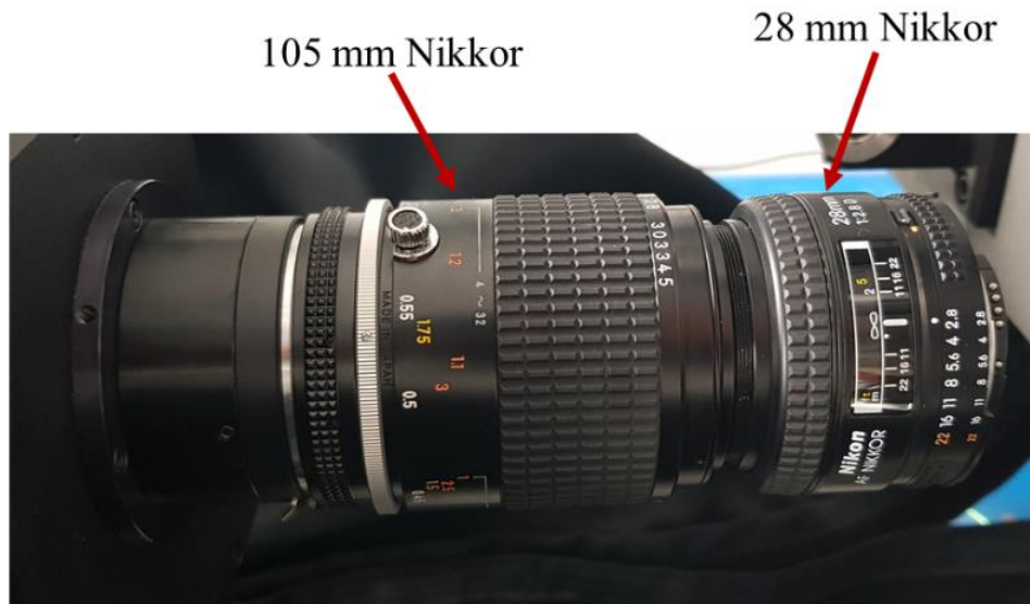
Figure 4.16. Optical collector mounted on the ICCD. In the picture, the IRO is on the left.
