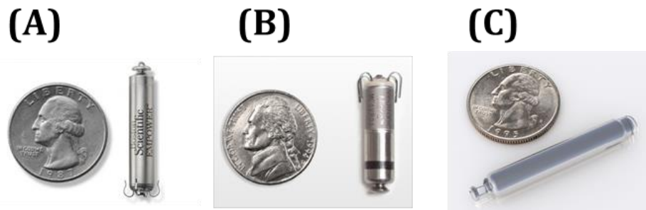
Figure 1-9: Leadless pacemakers: (A) Empower from Boston Scientific, (B) Micra leadless pacemaker from Medtronic, (C) Nanostim from St. Jude Medical
