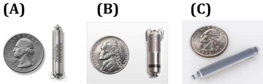
Figure 1-9: Leadless pacemakers: (A) Empower from Boston Scientific, (B) Micra leadless pacemaker from Medtronic, (C) Nanostim from St. Jude Medical
