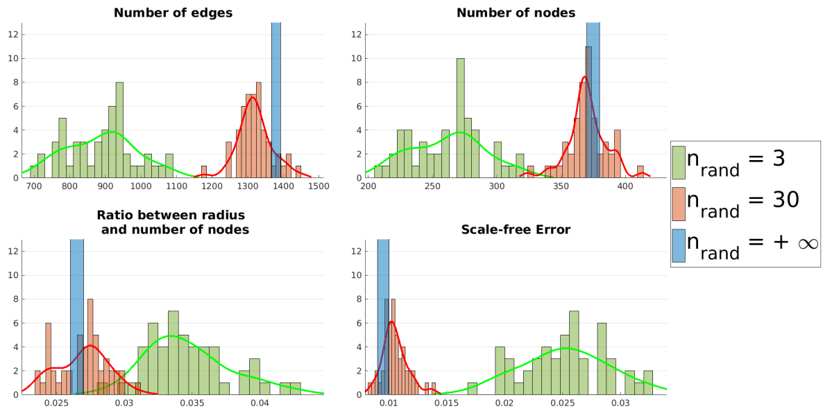
Figure 2.5: Histograms of the properties of the different networks obtained with different instances of the algorithm and with the same initial network. For each property, the x-axis represents the values and the y-axis, the frequency of apparition of each value. The green bars shows the values obtained when n_{\text{rand}} = 3 , the red bars when n_{\text{rand}} = 30 and the blue bar when n_{\text{rand}} = +\infty . The superimposed lines fits the histograms.
