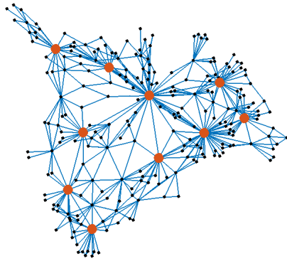
(a) Scale-free network. The ten most connected nodes are plotted in red.
