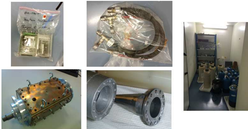
Figure 3.5: Examples of waste from the ARRONAX facility: electrical components, metallic activated pieces, vacuum pumps cables, liquids.
