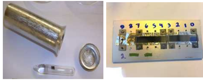
Figure 2.5: Pictures of the solid samples: example of sample in quartz ampoule before encapsulation for irradiation at ILL (left) and sample holder of ISOLDE SSP chamber with two Zn coated Au foils (right).
