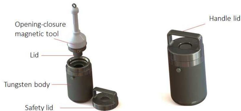
Figure 2.18: 3D drawing of the shielded container. The names of the principal elements are highlighted on the left image. The right image reports the closed configuration.
