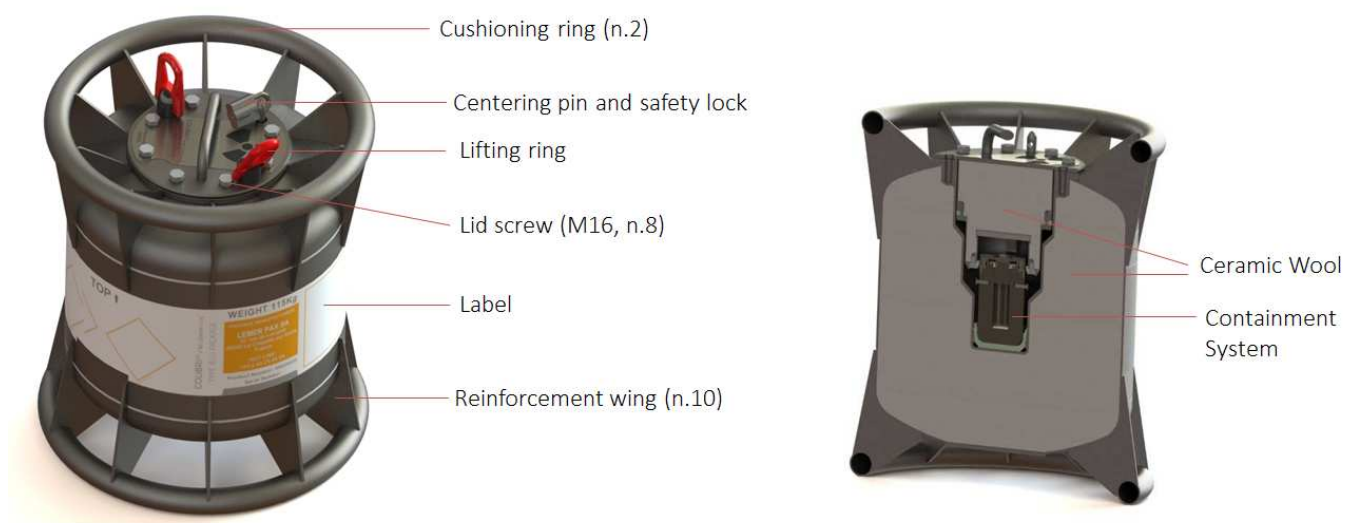
Figure 2.17: On the left side, a 3D drawing of the Overpack. The names of the principal elements are highlighted. On the right, a cut view of the package.
