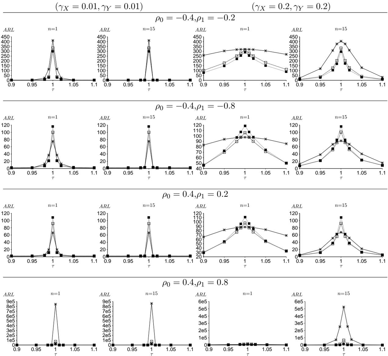
FIGURE 3.3 : Valeurs de  $ARL_1$  des cartes  $RRRZ_{2,3}$  ( $\square$ ),  $RRRZ_{3,4}$  ( $\blacksquare$ ) et Shewhart-RZ ( $*$ ) pour  $\gamma_X \in \{0.01, 0.2\}$ ,  $\gamma_Y \in \{0.01, 0.2\}$ ,  $\gamma_X = \gamma_Y$ ,  $(\rho_0, \rho_1) = \{(-0.4, -0.2), (-0.4, -0.8), (0.4, 0.2), (0.4, 0.8)\}$ ,  $\tau \in \{0.90, 0.95, 0.98, 0.99, 1.01, 1.02, 1.05, 1.10\}$ ,  $n \in \{1, 15\}$  et  $ARL_0 = 200$
