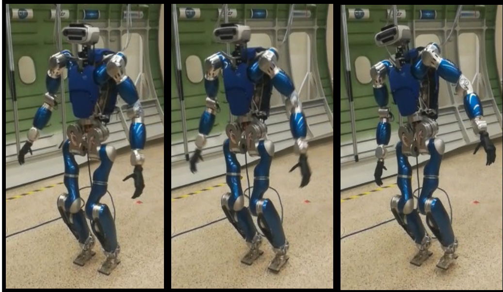
Figure 5.9: Emergency stop. Robot Toro triggering an emergency stop when the minimum allowed distance between arm and leg is reached.
