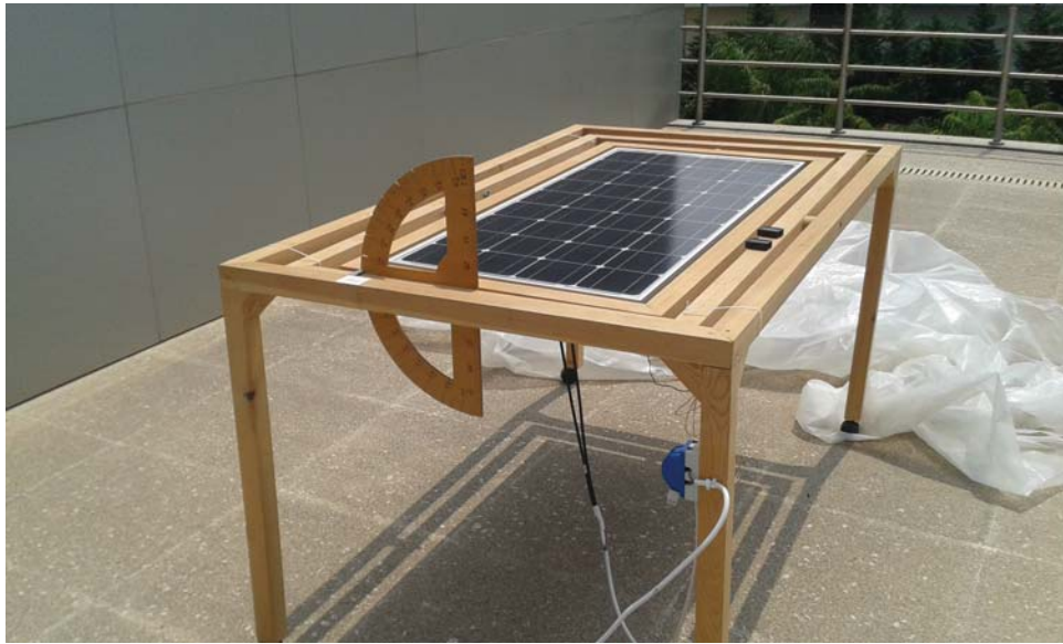
Figure 4.16: PV panel under real solar irradiance.
