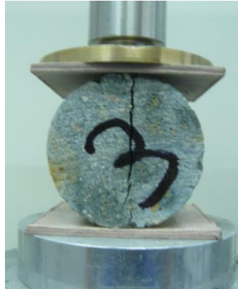
Figure 2-10 Set up for splitting tensile strength tests.
