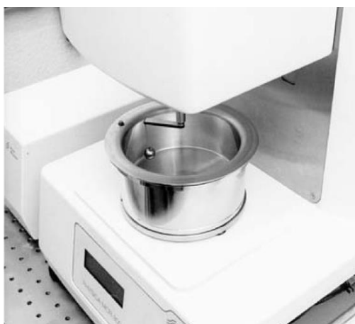
Figure 2-3 The BMS of Müller et al. (1999) implemented in a standard rheometer (Schatzmann et al., 2009).
