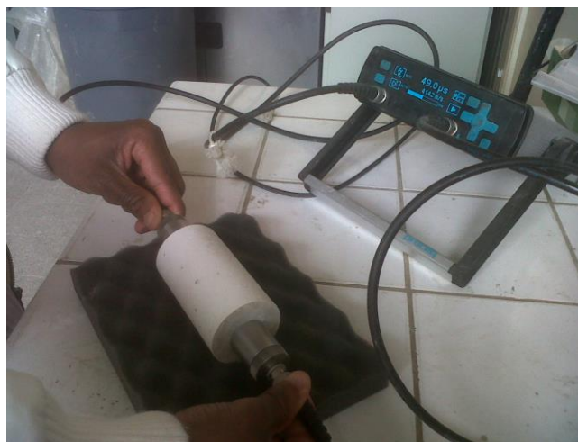
Figure 2-11 Set up for ultrasonic pulse wave velocity measurements.
