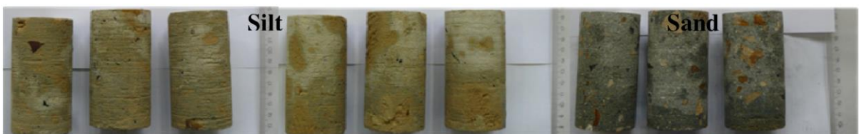
Figure 2-5 Cored specimens from block samples.
