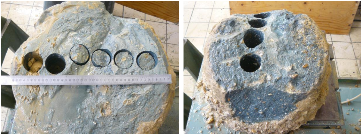
Figure 2-4 Coring of soil-cement specimens from block samples.
