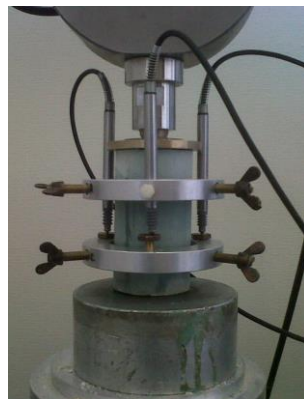
Figure 2-8 Set up for unconfined compression tests with local strain measurements.
