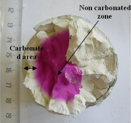
Figure 5-44 Carbonation depth of the treated soil specimens subjected to drying determined using a solution of phenolphthalein.
