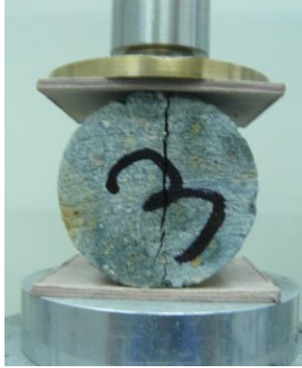
Figure 2-10 Set up for splitting tensile strength tests.
