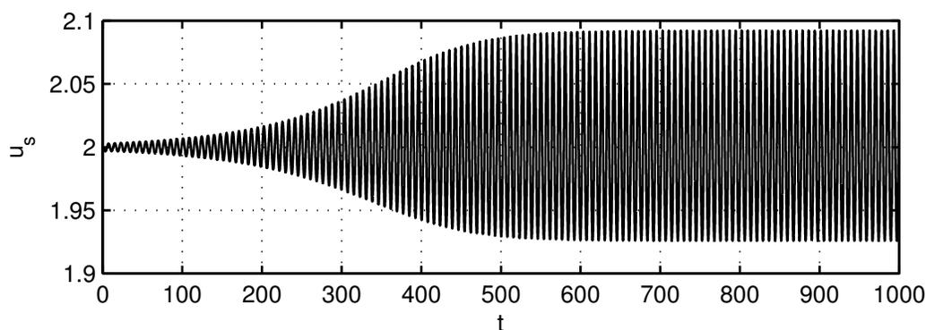
(b) Instability of the ZND solution and the limit-cycle attractor at  $\theta = 1.715 > \theta_c$ ,  $q = 1.7$ . Notice that the amplitude of the limit cycle scales roughly as the square root of the distance to the bifurcation point, as in a super-critical Hopf bifurcation.
