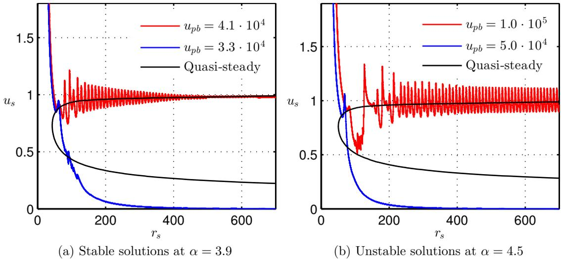
Figure 3.4: Initiation and failure for stable and unstable solutions. In both figures,  $\beta = 0.1$ , the length of the computational domain is  $L = 10^3$ , and the number of grid points used is  $N = 10^4$ .
