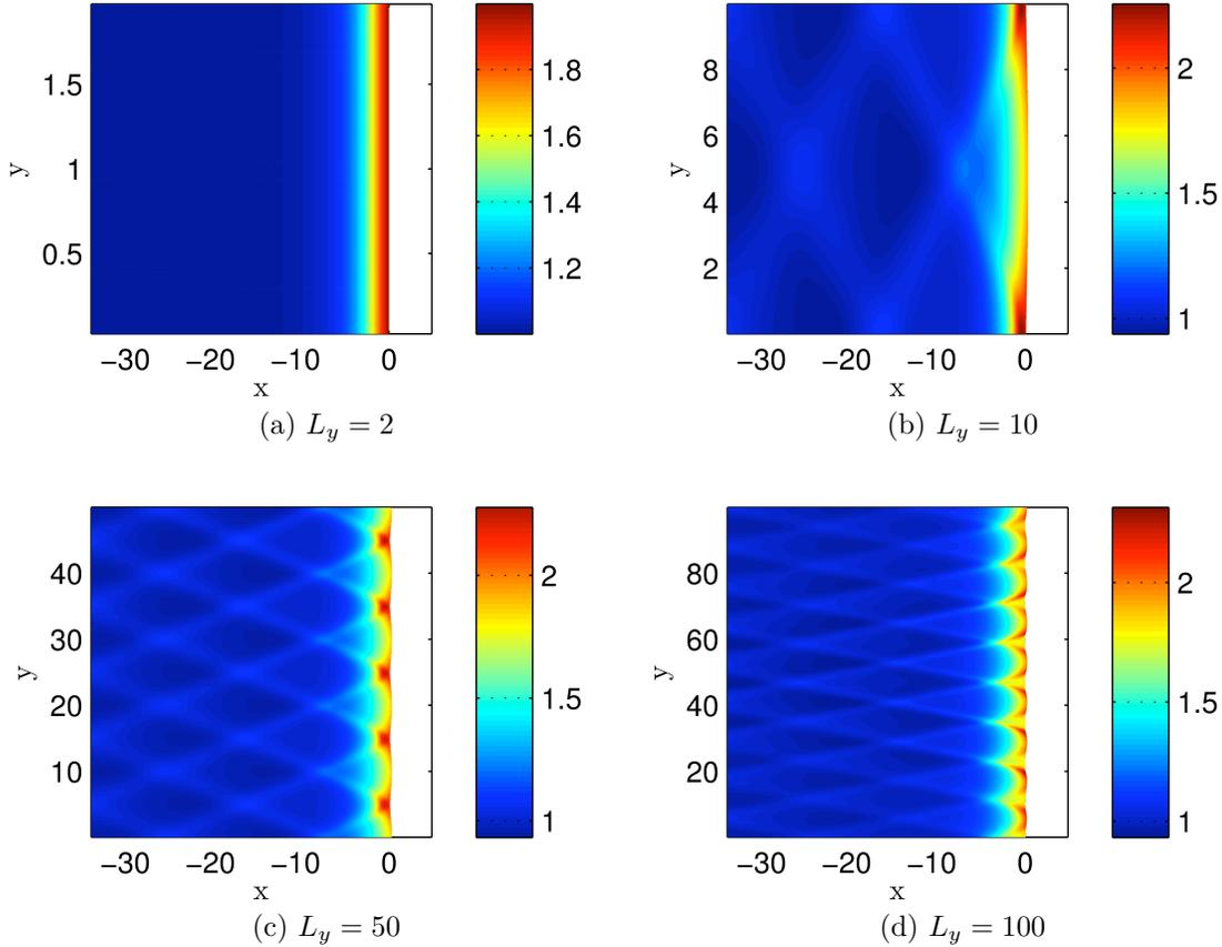
Figure 5.11: Dynamics of the asymptotic model in channels of different widths. The plots show the asymptotic variable  $u$ . The parameters are  $q = 1.7$ ,  $\theta = 1.65$ , as in Fig. 5.5. The white region corresponds to the ambient state ahead of the wave, with  $u = 0$ .
