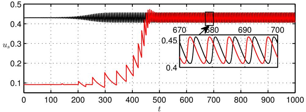
(b) At  $c_f = 0.125$ , the top branch is unstable. The integration is carried out starting both from the top branch (black curve) and the bottom branch (red curve). The pulsating instability is due purely to the presence of friction.
