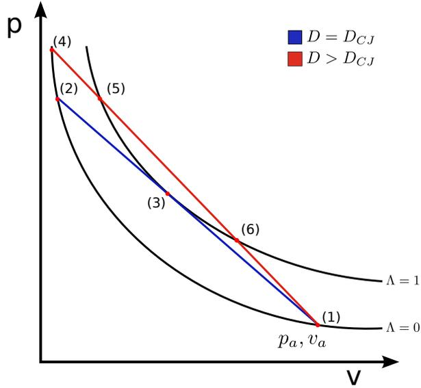
Figure 1.3: ZND wave diagram. The black curves represent the Hugoniot curves for  $\Lambda = 0$  and  $\Lambda = 1$ , and the colored straight lines are the Rayleigh-Mikhelson lines for the Chapman-Jouguet and overdriven cases.
