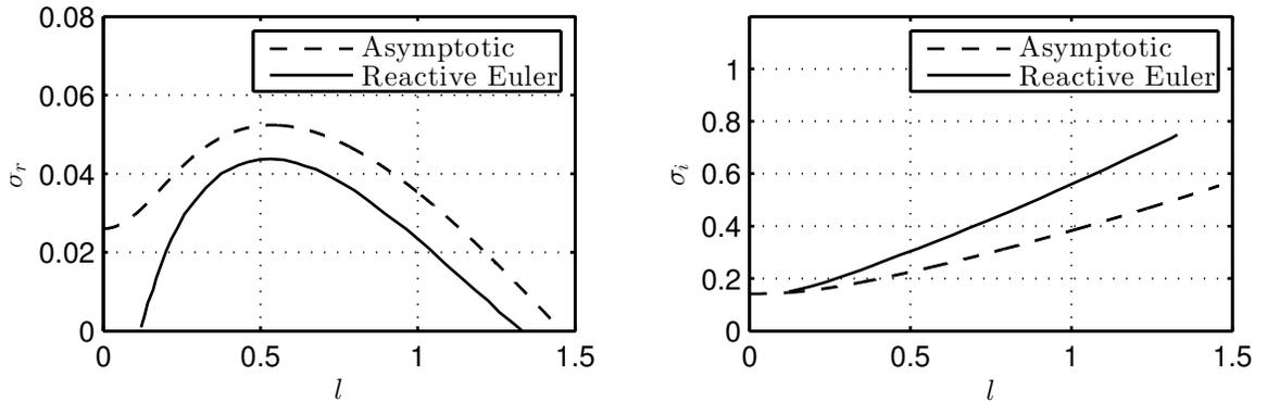
Figure 5.6: Comparisons of the growth rate and frequency for the most unstable mode versus the wave number, for  $Q = 0.4$  and  $E = 50$ . The dashed curve corresponds to the model in this paper. The solid line corresponds to the reactive Euler equations as computed in [1].
