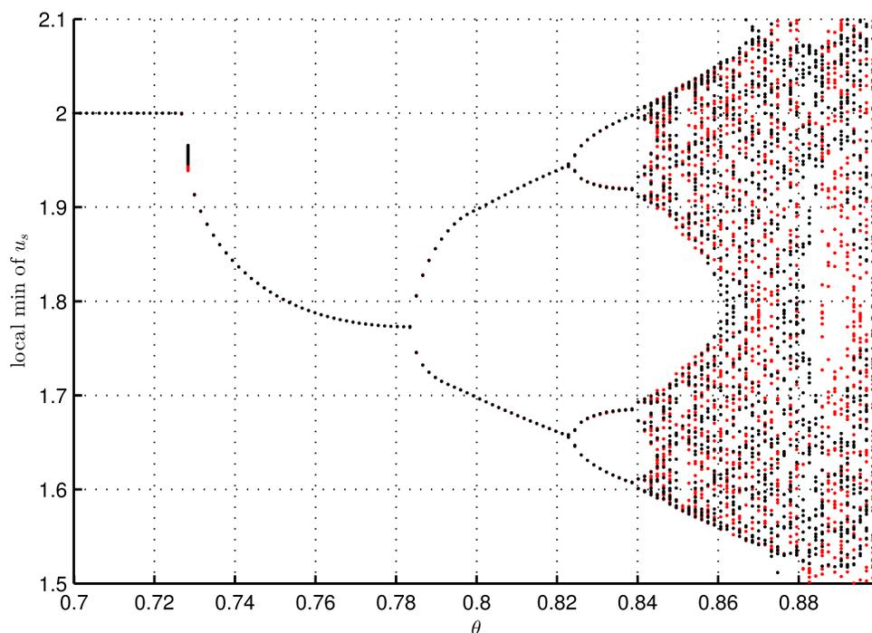
Figure 5.10: The bifurcation diagram at  $q = 5$  showing the local minima of the attractor solution's shock value,  $u_s(\tau) = u(0, \tau)$ , as a function of the dimensionless activation energy,  $\theta$ . The simulations were carried out at two different resolutions:  $N = 15,000$  (red) and  $N = 30,000$  (black) grid points on the computational domain of length  $L = 30$ . We see that away from the chaotic regimes, the predictions are nearly identical.
