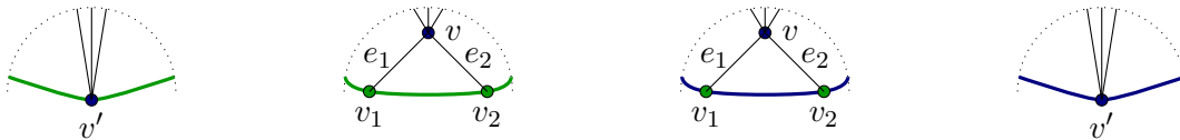
Figure 4.42: On the center, the two possible configurations for a \lambda , on the sides, the D -graphs G' obtained from G .
