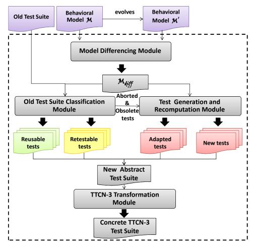
Figure 4.1: TestGenApp: Selective test case generation approach.
