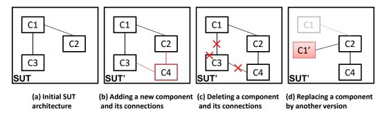
Figure 2.2: Basic structural reconfiguration actions.
