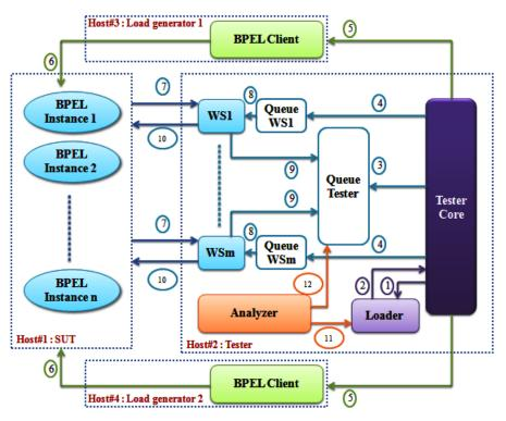
Figure 8.2: Load Testing Architecture.
