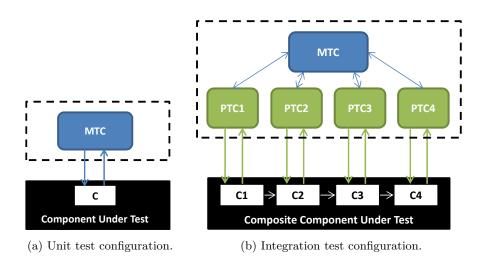
Figure 3.4: TTCN-3 test configuration for unit and integration testing.
