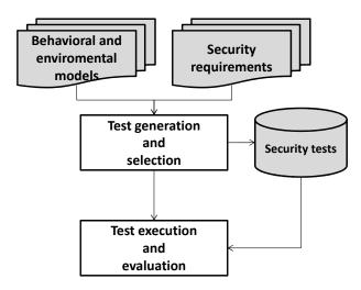
Figure 11.1: Model based security testing process.
