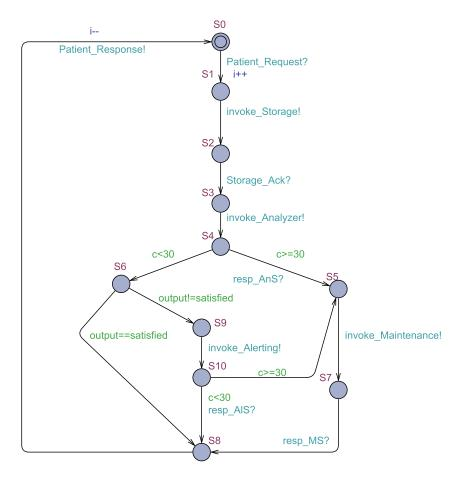
Figure 7.12: The TRMCS process modeled in Timed Automata.
