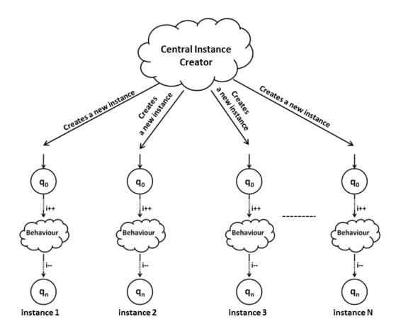
Figure 7.7: A central instance of the SUT is in charge of creating new instances.
