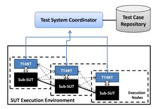
Figure 3.7: The distributed test execution platform.
