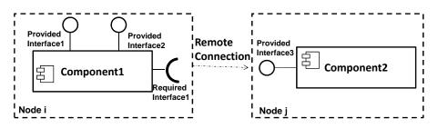
Figure 2.1: Distributed component-based architecture.
