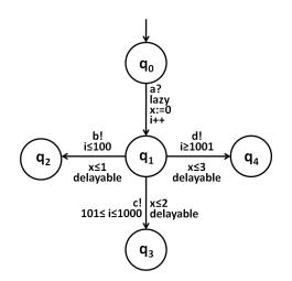
Figure 7.3: An example where the SUT produces different output actions depending on the current load.
