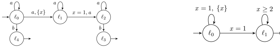
Figure 9.5: Examples of determinizable TAs not treatable by (3).
