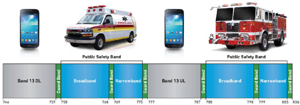
FIGURE 1.2: Portion example of the segmented spectrum with tiny separation bands. Source [Mil15a].
