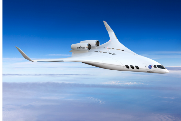
Figure 1.16: Rendering of the BWB Ascent 1000, announced by DZYNE and expected to fly in the near future [PSY18].
