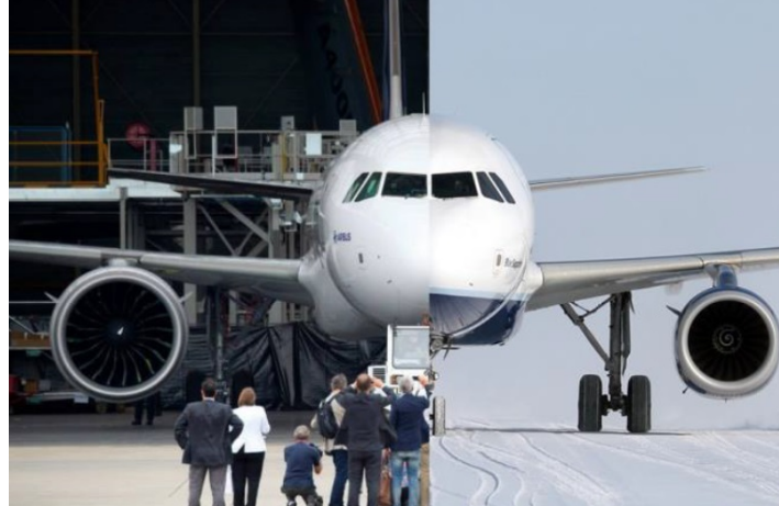
Figure 1.7: Comparison between the Airbus A320 (right) and the new A320 Neo (left) mounting the innovative LEAP engine.
