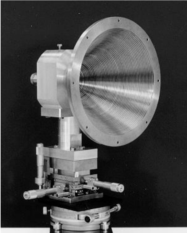
Fig. 4. Fabricated corrugated horn. The external diameter of the antenna is about 250 mm and the total length is 257 mm.
