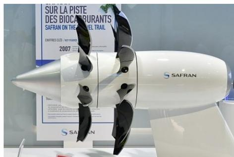
(b) Open Rotor Safran Aircraft Engines
