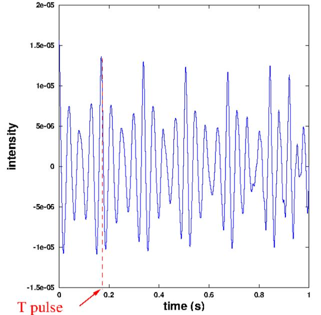
FIG. 5. Graph of the auto-correlation  $C_{T_{signal}, T_s}(\tau)$  of unit *C* : the maximum of correlation for  $T_{pulse} \simeq 0.17$  s corresponds to a frequency  $f_{pulse} \simeq 6$  Hz. The time  $T_{signal}$  is 4 s. (color online)
