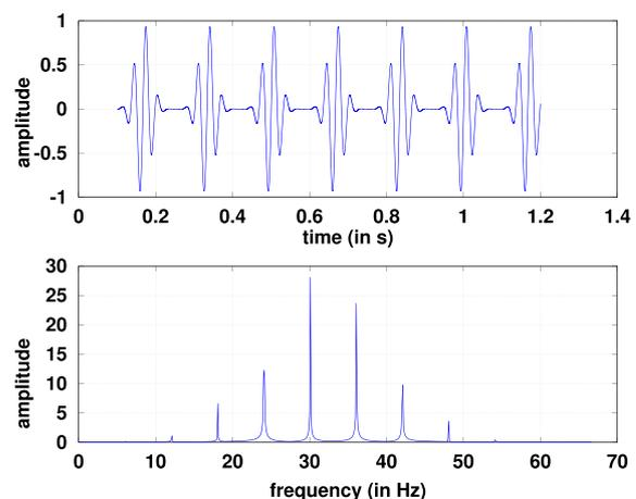
FIG. 3. (Color online) Model A in waveform (top) and its FFT (bottom). In model A, we choose the pulse as the product of a sine function of frequency  $f_0 = 31.7$  Hz with a Gaussian of standard deviation ( $\sigma = 0.02$  s). We also choose  $f_{\text{pulse}} = 6$  Hz. In the FFT we can see that the peaks are multiples of  $f_{\text{pulse}} = 6$  Hz.
