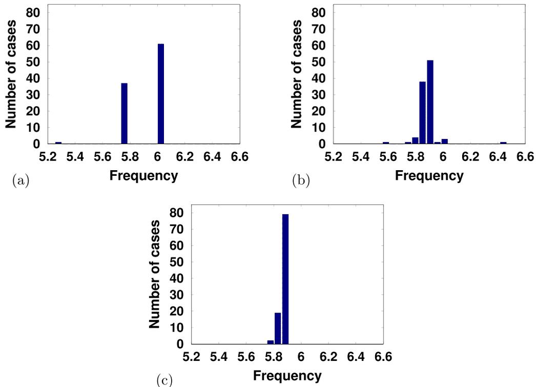
FIG. 7. (Color online) Histograms of the estimation of pulse rate  $f_{\text{pulse}}$  for unit  $C$  of 100 high SNR blue whale phrases. Three different methods of estimation were employed. (a) Estimation by difference of frequency peaks  $f_i$  in the FFT. (b) Estimation by summed autocorrelation of the envelope of the signal. (c) Estimation by summed autocorrelation of the signal.
