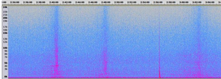
Figure 12: Sounds of the boat (at 2h40, 2h48 and 3h02) around an explosion (at 2h56)
