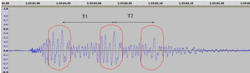
Figure 5: Explosions recorded in Chañaral in wave form and bubble pulse period  $T_i$
