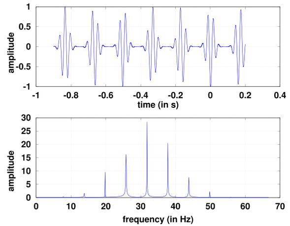
FIG. 4. (Color online) Model B in waveform (top) and its FFT (bottom). In this model, we choose the tonal function  $g_{T_0}$  as a pure sine function of period  $T_0$  and the envelope  $e$  as a Gaussian with standard deviation  $\sigma = 0.02$  s. As in Fig. 3, we choose  $f_0 = 31.7$  Hz and  $f_{\text{pulse}} = 6$  Hz. In the FFT we can see that the frequency peaks are not centered at multiples of  $f_{\text{pulse}}$ .
