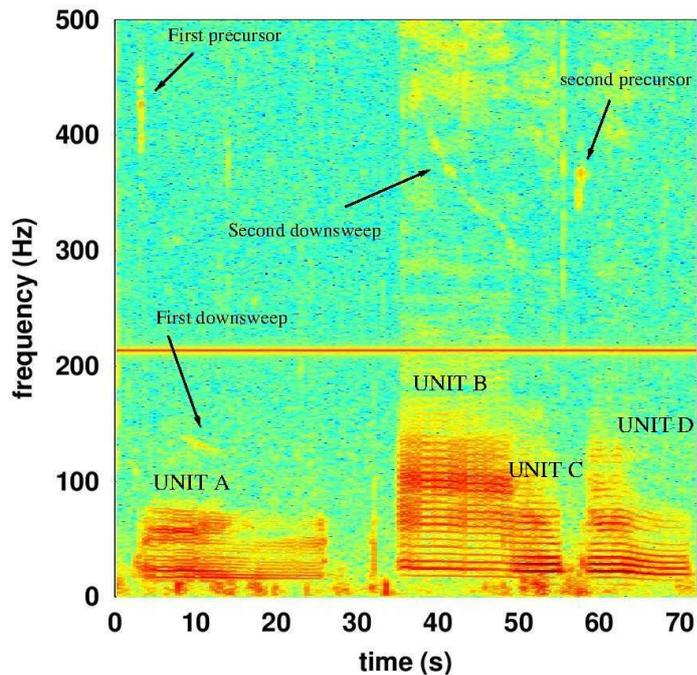
Figure 3 : Time frequency representation of a SEP2 song recorded off Isla Chañaral, the 2nd of february 2017 (Fast Fourier transform, Blackman window of 65536 points, overlapping 75%) using Octave software (Eaton et al. 2009). The line at 213 Hz is a constant electronic noise coming from the coupling between the hydrophone and the recording device. Units A,B,C,D are clearly visible as well as precursors and downsweeps belonging to the song.
