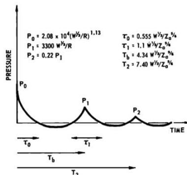
FIG. 1. Sketch of pressure versus time waveform of an explosive source at short ranges. Formulae are from Gaspin and Shuler.<sup>3</sup>  $W$  is source weight in pounds of TNT;  $Z_a$  is depth in feet, plus 33; pressures are in psi; times are in seconds.
