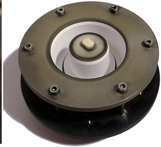
(b) The ISCT200-MS Hall thruster (shielded)
