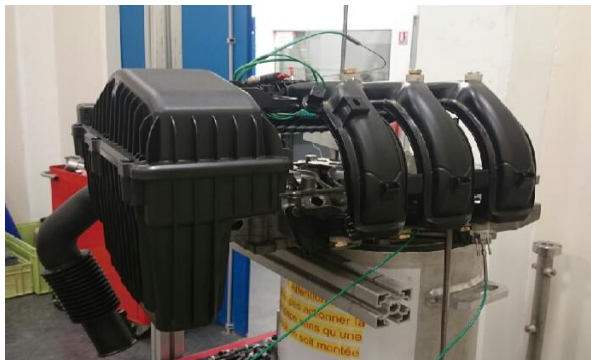
Figure II-19 – DFB tests on EB2 intake system
