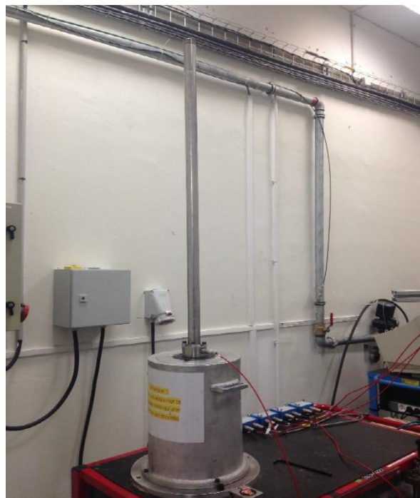
IV-17 - Dynamic flow bench test on a tube (L=1086 mm, D=30 mm)
