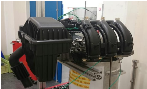
Figure II-19 – DFB tests on EB2 intake system
