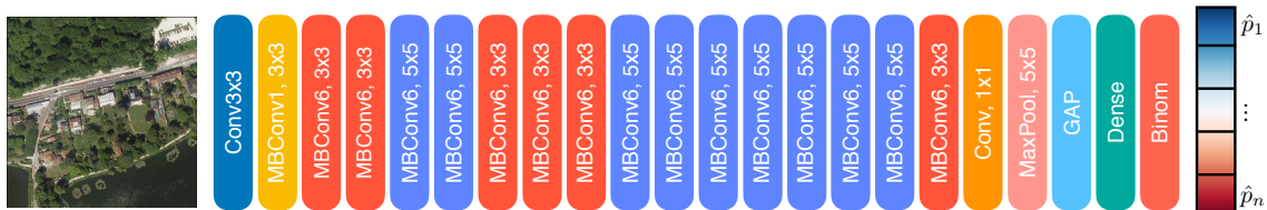
Figure 5-2: Model Architecture: The model takes the aerial tile as an input which is then fed through several MBConv blocks. The feature maps end up going through a global average pooling layer and a dense layer to output a single value p . From it, probabilities for each socioeconomic class are generated from a binomial distribution B_{(N_{SES}, p)}
