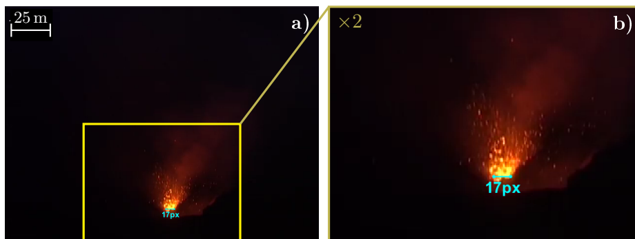
Figure 2.9 – Measurement of the diameter of the conduit at Yasur (June, 2009). The gas pocket, surrounding by magma is 17 px width just before it explodes. The diameter of the conduit is 5.1 m for a scale of 30.5 cm.px -1 .
