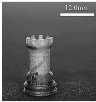
Figure 2.5 Chess rook fabricated in stereolithography from epoxy/carbon nanotubes mixture [89]
