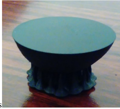
Figure 2.27 A failed attempt to manufacture a full acrylate with carbon spheres. Only a quart of the sphere was manufactured
