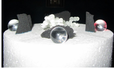
Figure 3.29 The alignment procedure showing the aggregate AG_{005} on the expanded polystyrene holder with the dielectric alignment spheres
