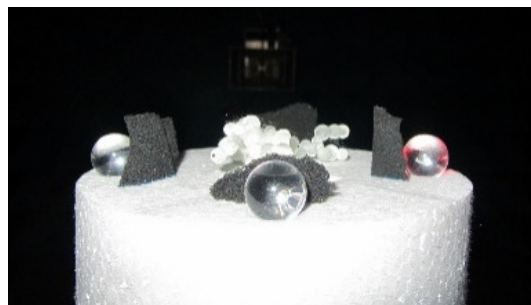
Figure 1.28 A photo of a polystyrene holder made especially to the alignment of a soot aggregate analog of complex shape. The dielectric spheres and the black absorbing pieces are removed after the alignment is accomplished
