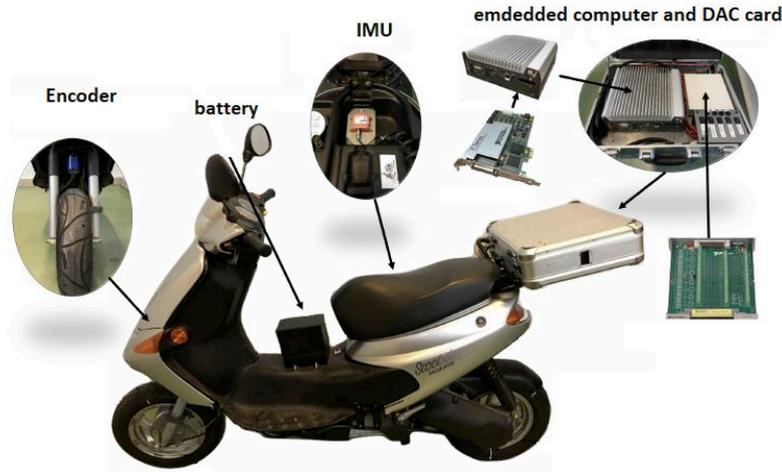
FIGURE 2.20: Instrumented Scooter at the IBISC Lab, university of Evry.
