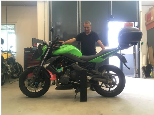
FIGURE 3.5: The instrumented Kawasaki ER6N PTWV.
