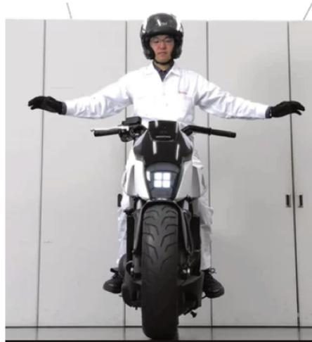
FIGURE 1.7: Honda's self-balancing motorcycle (Honda, 2017)
