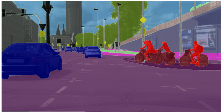
Figure 3.2: Image frame taken from Cityscapes Dataset showing image pixels classified according to object class to which they belong. The image corresponds to the city of Cologne, Germany.
