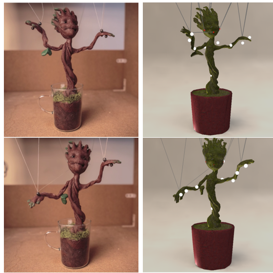
Figure 3.26: A puppet representing the character Baby Groot, actuated by 12 cables going through the hands and head and. Left: the inverse simulation. The white spheres represent the keypoints target. Right: the real prototype controlled by the simulation.
