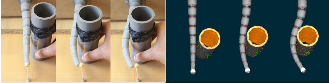
Figure 4.17: Top: Real cable-driven soft robot, Bottom: Corresponding motion computed by the simulated inverse model. We interactively move an obstacle while the input of the inverse model is a fixed position of the robot's tip.
