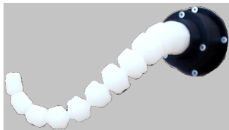
Figure 3.18: Soft trunk #2. Second design for grasping tasks.
