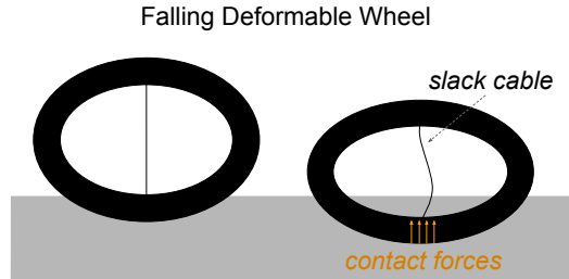
Figure 5.2: Example where a cable can not remain straight. In such cases, the cable constraint (i.e. limit on displacement) is removed from the optimization problem, for a certain amount of time that corresponds to the time it takes to the motors to pull on the cable.
