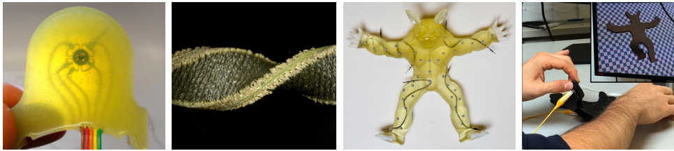
Figure 1.11: (left) Force sensor using embedded micro-fluidic channels from (Vogt et al. 2013). (middle) Silicone textile composite capacitive strain sensor from (Atalay et al. 2017). (right) Defsense, deformable input devices from (Bächer et al. 2016)
