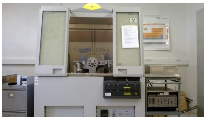
Figure II. 2. Diffractomètre PANalytical X'Pert Pro
