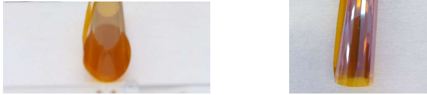
Figure 2-11. Effect over Kapton 25µm after deposited the \mu\text{C-Si} .
