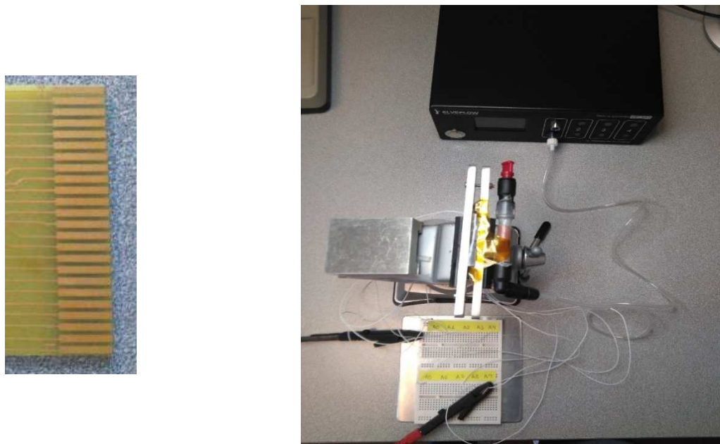
Figure 4.5 Board card of resin with printed electrodes and final system with the sensors connected to the board card.
