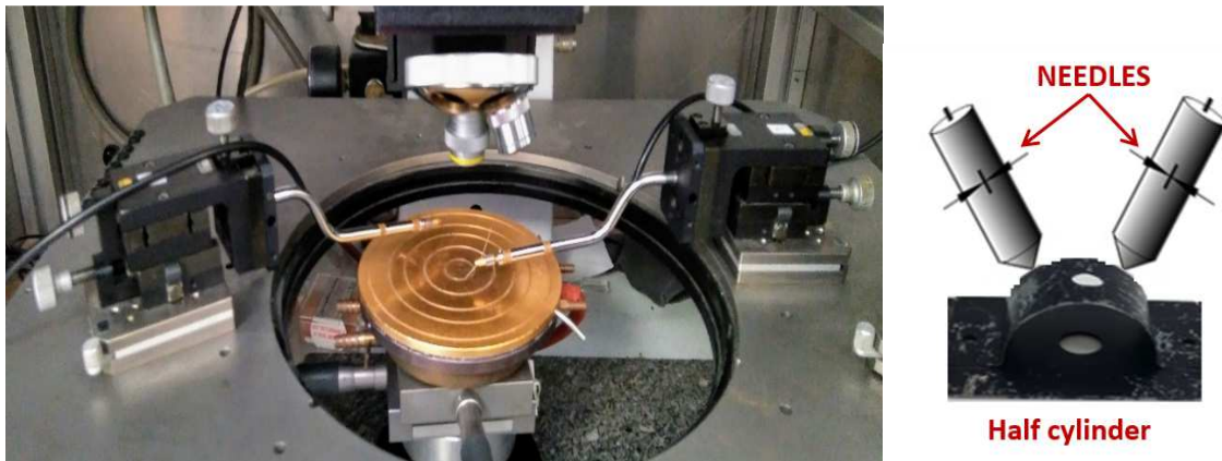
Figure 4.2 Characterization system based on probes with needles to perform static deformations.
