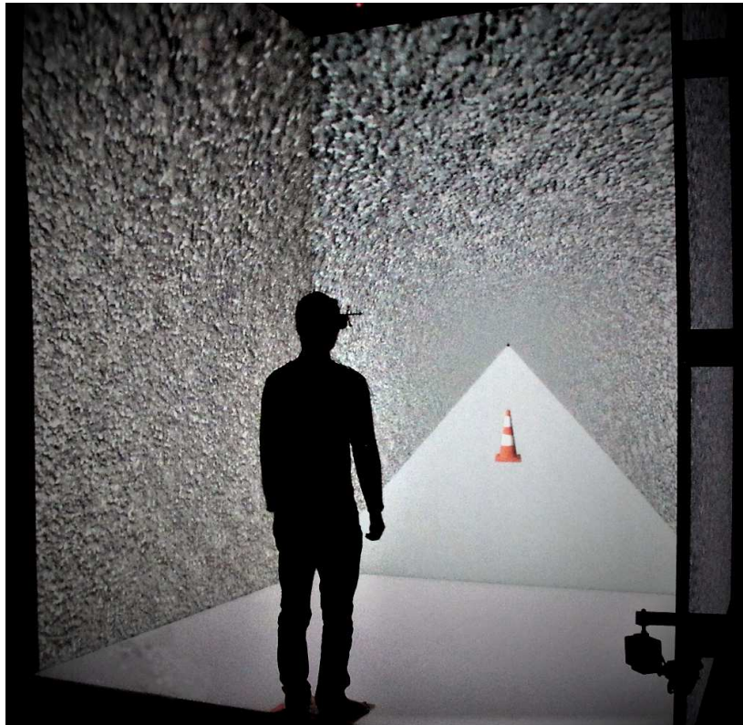
Figure 2.1 – The experimental set-up. The large screen immersive display (CAVE) at Aix-Marseille University.
