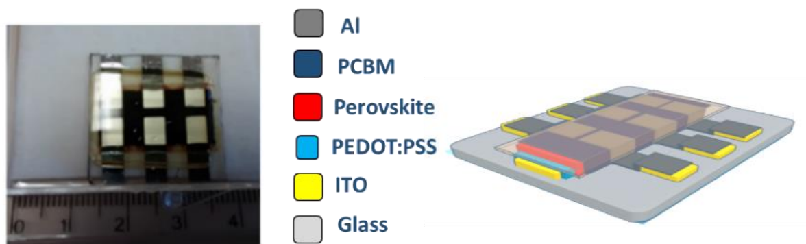
Figure 5.4. Device architecture of the inverted perovskite solar cells used in this study.
