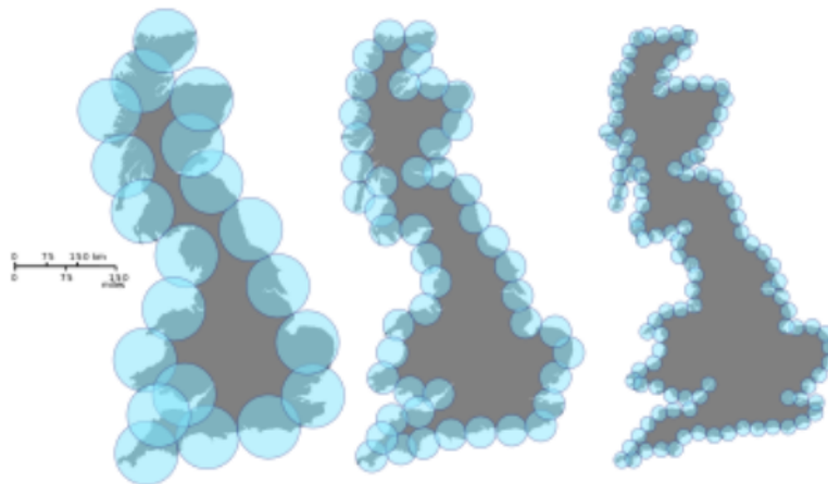
FIGURE 2.8: Illustration of the Hausdorff dimension concept applied to the Great Britain coastline example. Image taken from Wikipedia.
