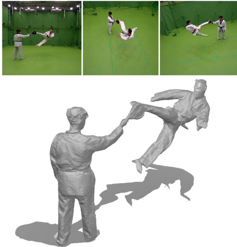
Figure 1.6: A challenging dynamic scene with fast motions and a mid-scale acquisition space, hence low image resolution on shapes in addition to motion blur and occultations. Temporal integration helps recovering highly detailed models.
