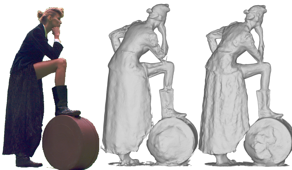
Figure 3.9: Challenging scene captured with a passive RGB multi-camera setup [5]. ( left ) one input image, ( center ) reconstructions obtained with classical 2D features [74], ( right ) proposed solution. Our results validate the key improvement of a CNN-learned disparity to MVS for performance capture scenarios. Results particularly improve in noisy, very low contrast and low textured regions such as the arm, the leg or even the black skirt folds, which can be better seen in a brightened version of the picture in Figure 6.5.
